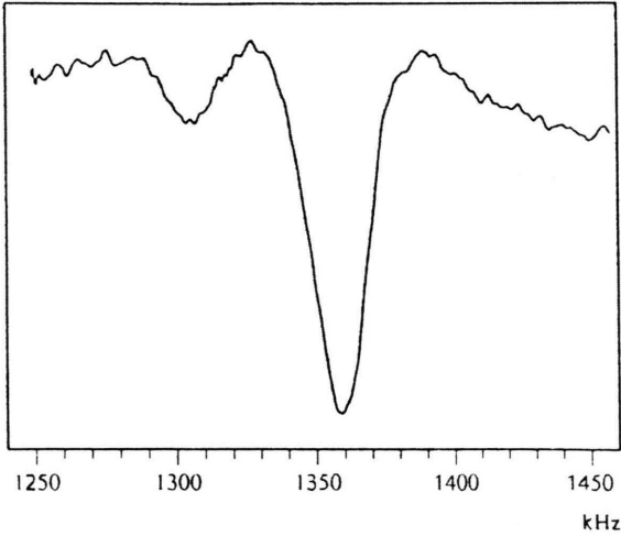
Fig. 23. ^{11}\text{B} NQR responses from vitreous \text{B}_2\text{O}_3 .
